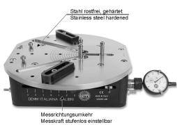
Reversible measuring direction Adjustable measuring force
