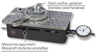
Reversible measuring direction Adjustable measuring force
