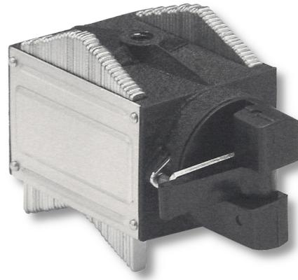
**Product description****Delivered in individual packages****Technical Data****Size:** 91x52x55mm/M8**Article no.:** 1400748x**Brand:** FISSO**Manufacturer number:** 5.088**Adhesive force:** 600N**Size:** 91x52x55mm**Switchable:** Yes**Thread:** M8**Type:** Anyform magnet**Weight:** 0.96kg
