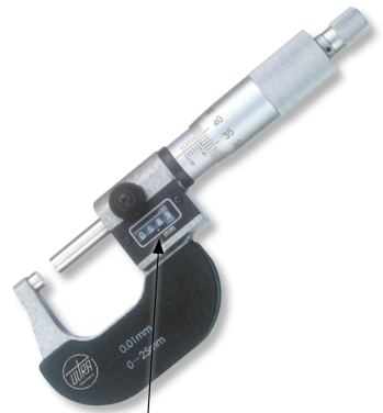
Ablesung 0,01mm am Fenster Reading 0.01mm at window
