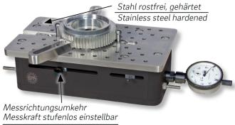
Reversible measuring direction Adjustable measuring force
